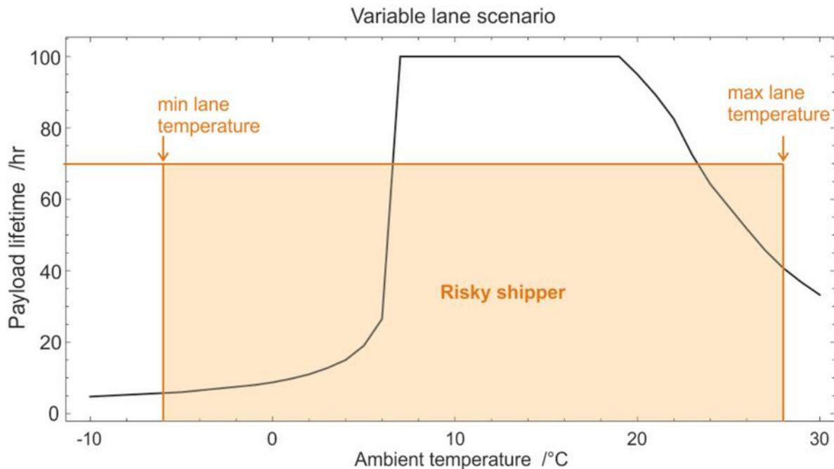
Figure 4: Spread of lane temperatures is significantly wider than sweet spot of performance curve. Shipper is considered risky for this lane. Black line – performance curve; orange lines – lane characteristics.
