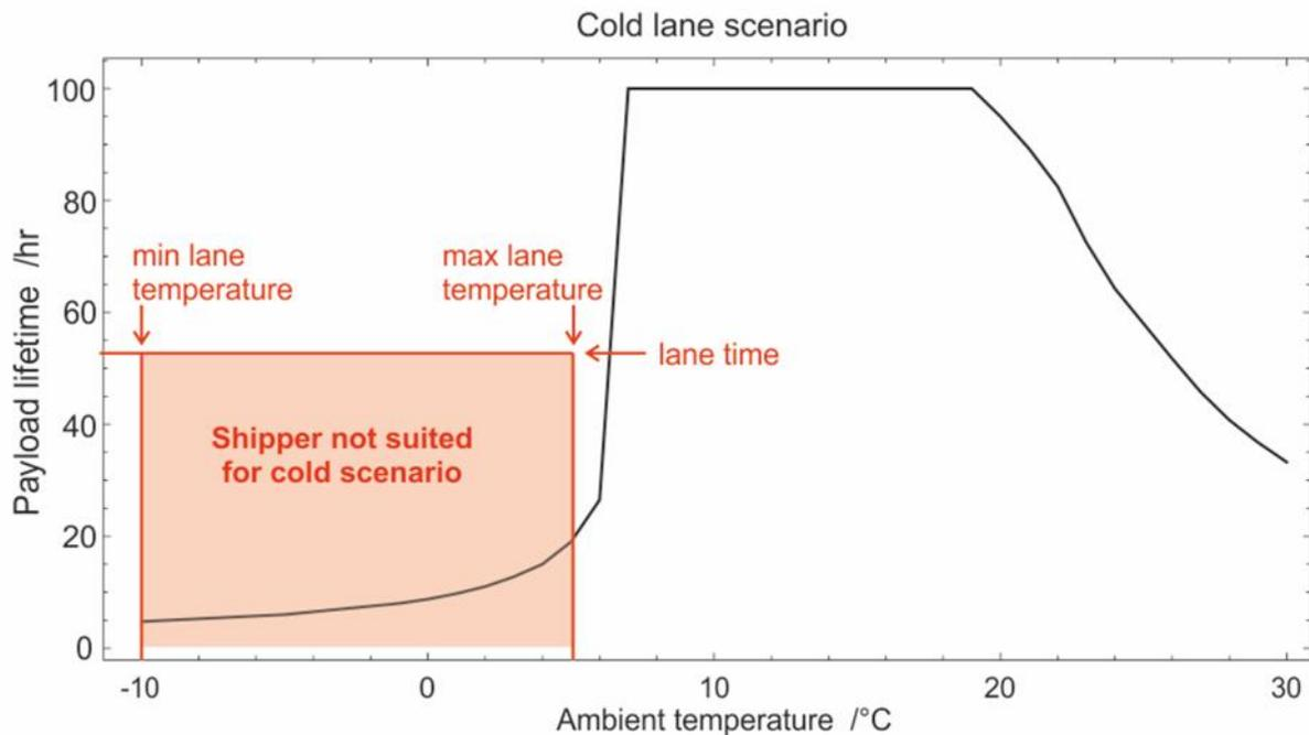
Figure 3: Lane temperature exceeds performance curve for the planned lane time of 52 hours, indicating that shipper is not suited for the “cold lane” scenario. Black line – performance curve; red lines – lane characteristics.
