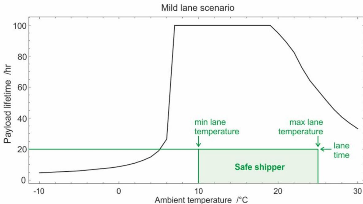
Figure 2: Lane temperature is within performance curve for the entire lane time, indicating that the shipper is a safe choice for this lane. Black line – performance curve; green lines – lane characteristics.
