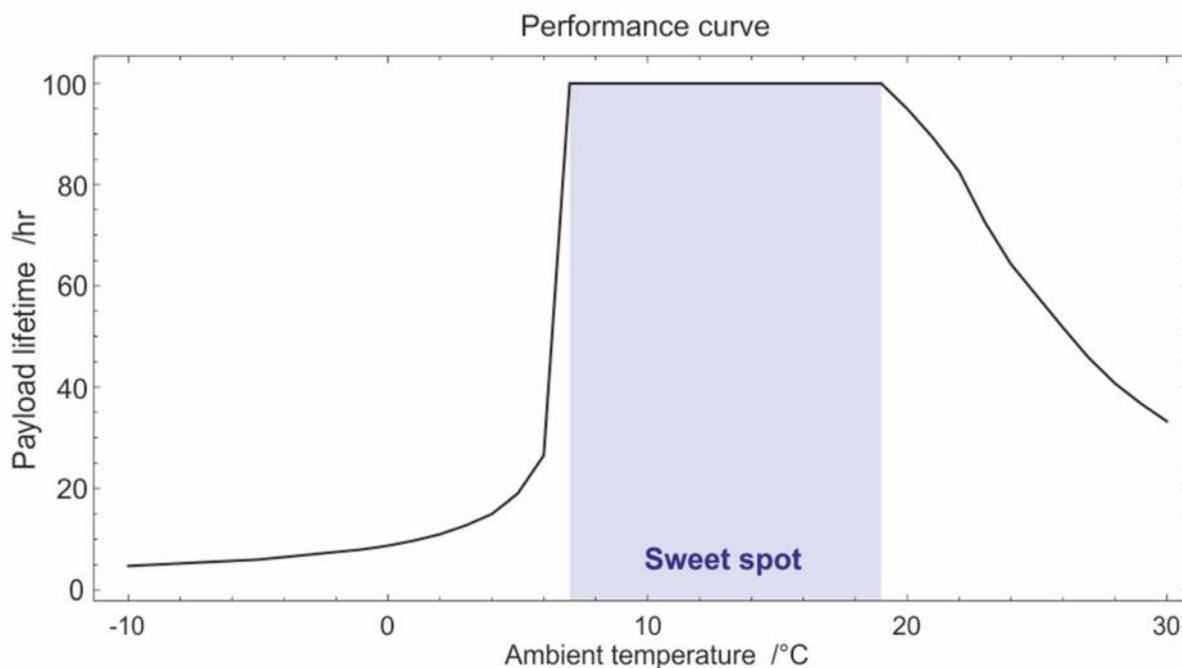
Figure 1: The performance curve represents the lifetime of a temperature-sensitive payload for a shipper as function of ambient temperature. Maximum lifetime is capped at 100 hours. Solid black line – performance curve; blue area – “sweet spot”, i.e. ambient temperature range where shipper performance is optimal.
